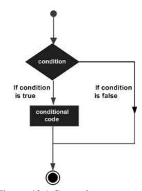
Figure 13.1 Control structure
